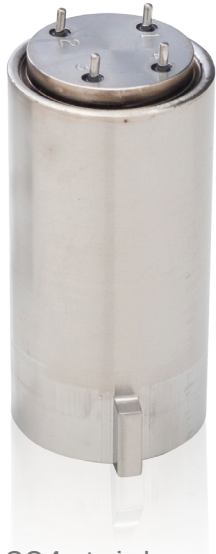
Case and header 304 stainless steel, terminal nickel iron alloy hot soldered
