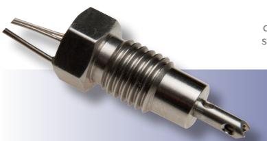
The 1SE601 is a pyrotechnic actuated cutter specifically designed to puncture a steel disc and release gas from a cylinder through the hollow piston.
