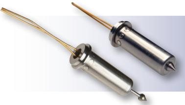
It is used as an electrically activated system to penetrate bursts discs. The 1MT171 Piston Actuator is a completely self-contained, non-sealed electroexplosive device. The hardness of the pointed piston is 220 Bn. The leads are copper cored and gold plated.
