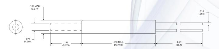
FOR 1MT11, BODY LENGTH IS .530 INCH (13.462) AND STROKE LENGTH IS .125 INCH (3.175)  $\mbox{DIMENSIONS IN ( ) ARE IN MM}$
